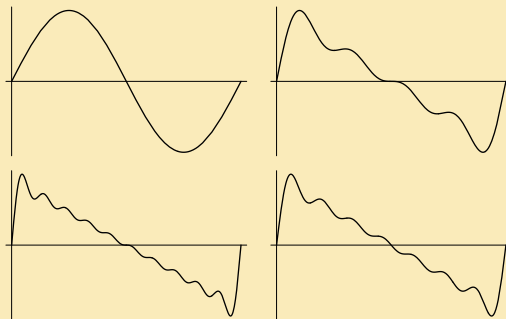
Figure 9.7. Graph of \sum_{k=1}^n (\sin k\theta)/k on [0, 2\pi] for, clockwise from upper left, n = 1, 4, 7, and 10 .
