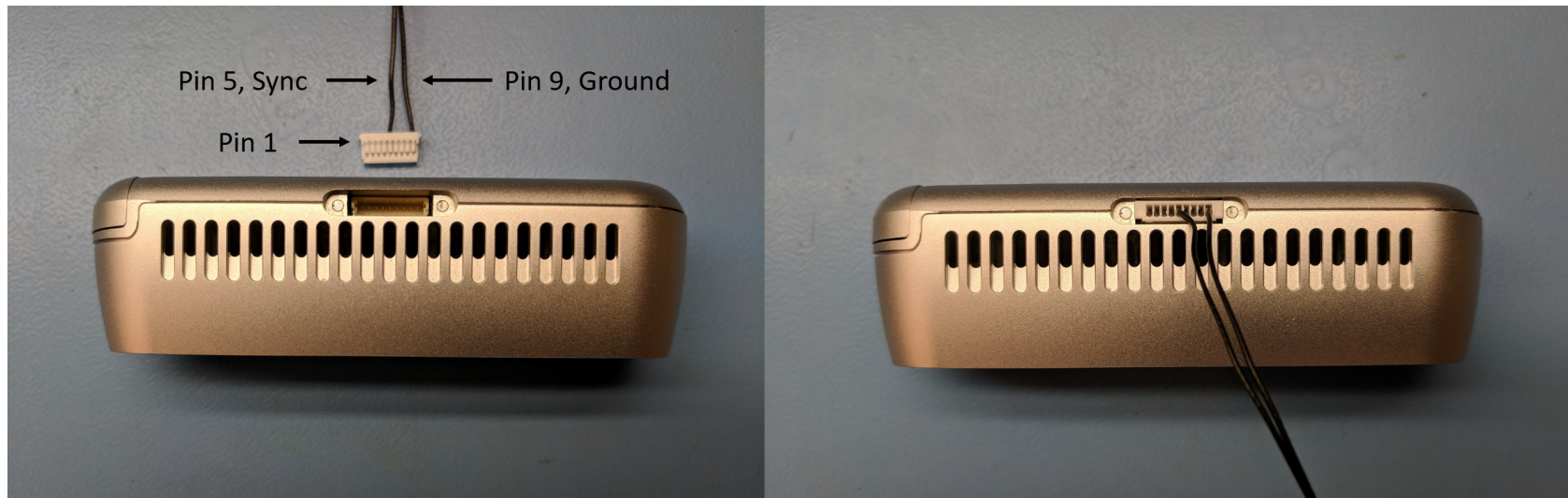
Figure 3. Connector a sync cable to the D435.
