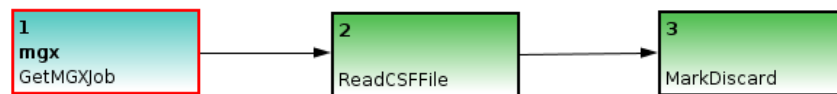
Figure 3.6: A minimal working example of a pipeline developed for MGX, which would set the discard flag for all sequences.
