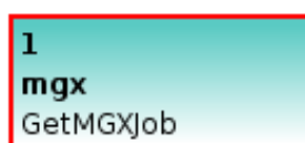
Figure 3.4: The GetMGXJob node provides necessary context for executing a workflow within MGX, such as database access. By convention, this node has to be named mgx .
