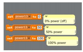
"Set power13 to 0" is the same as "broadcast pin13off" and "Set power13 to 100" is the same as "broadcast pin13on"
