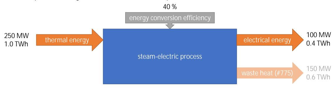
A steam-electric process is an energy transformation that converts thermal energy to electrical energy. A steam turbine and an electro motive generator are participating in a steam-electric process.
