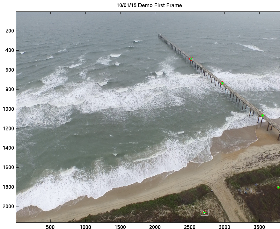
Figure 1. First frame of demo video showing the identified gcps (green asterisks show the five locations clicked by the user – gcps [1 2 3 6 7] in inputs.gcpList) and the best fit locations from the fit (red circles). The first gcp (seaward on the pier) is a tiny white point that is hard to see. The white square surrounding the bottom gcp indicates the selected sampling region for the automatic reference point search for this target (Figure 2).
