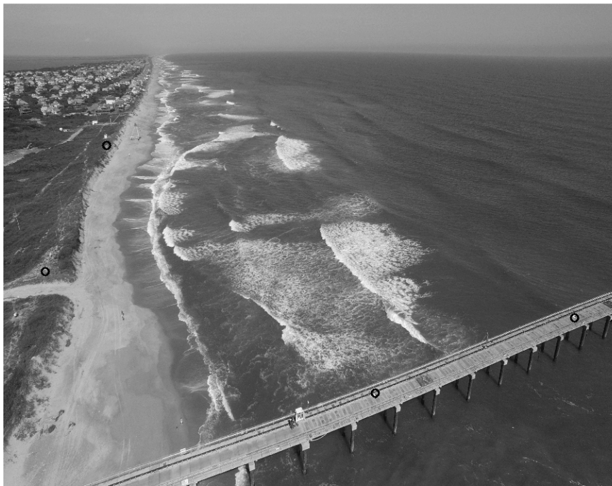
Figure 2. Example snapshot used in testing the accuracy of GPS metadata. The four selected GCP locations are shown by black circles.
