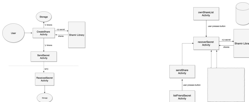
(a) Graph presenting data flow through the system (b) Graph presenting data flow through the system during recovery
