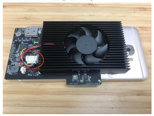
7) Once the fan has been disconnected, remove the old heatsink. Clean the thermal paste on the back of the phone. Reapply thermal paste to the back of the new heatsink before reattaching to the phone. Leave a gap around the edge to allow the thermal paste to spread. (Alternatively, you could reclaim the thermal paste on the phone and old heatsink and add to the new heatsink).
