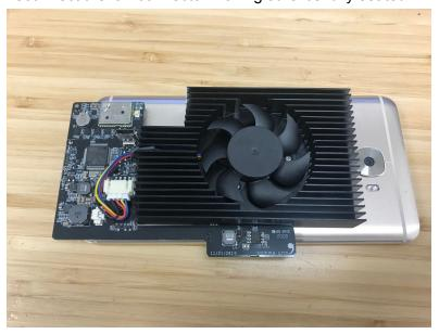
9) Reassemble the comma two in the opposite order paying attention to the IR LEDs and GPS antenna wire.
