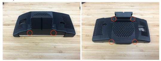
2) Carefully remove the "bottom" piece from the device.
