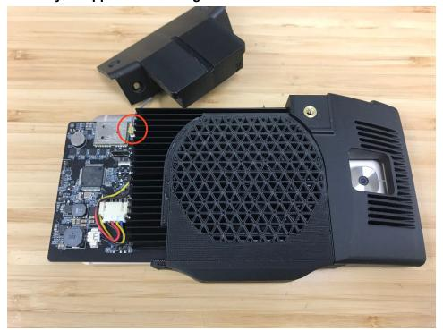
4) Remove the "Top" piece by sliding it off
