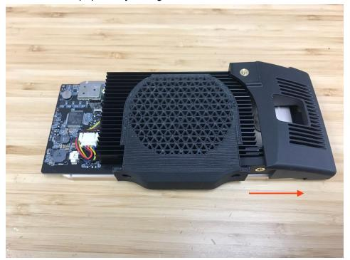
5) Remove the back piece by gently removing the piece from the top part first. Once the top piece is removed from the heatsink, gently remove the bottom part. Pay attention to the IR LEDs (Circled in red) as you can damage if you are not careful.
