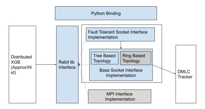
Rabit is featured with simplicity in design and implement based on C++ socket. It's base socket interface implementation provides *non fault tolerant, best effort, pull based* socket implementation of *init, shutdown, allreduce, broadcast, getworld, getrank* etc MPI interface implementations.
