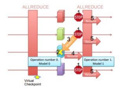
In case of fault recovery phase, it runs 5 steps process to recover failed node(s)
