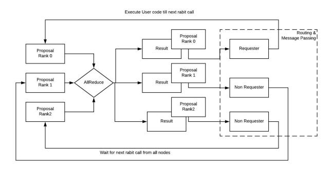
Following diagram shows a simplified version of how rabit consensus protocol helps failed node catch up with the rest in a rabit program lifecycle.
