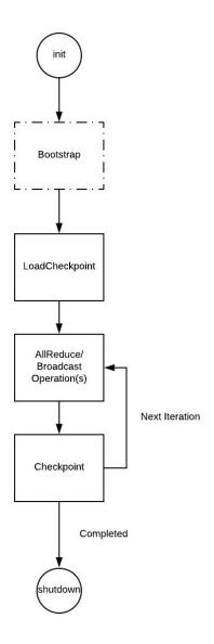
Rabit was implemented in C++ with multiple platforms support. It also provide Python/C binding for user to interact with Python code or JVM JNI code. With dmlc tracker (Python) to coordinate registration and binary tree topology setup, Rabit cluster form tree shaped network topology to facilitate collective allreduce/broadcast/loadcheckpoint/checkpoint etc operations.
