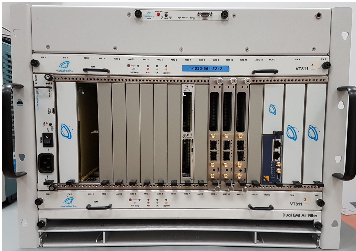
Figure 1: Micro TCA chassis with 3 Sayma AMC modules inserted
