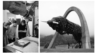
Figure 1 Robot setup at Snøhetta during a KUKA | prc workshop (left); Red Bull Arch at the Formula 1 track in Austria (right). Eighty-three positive molds for the aluminum arch fabricated with a used robot via KUKA | prc and Grasshopper.
