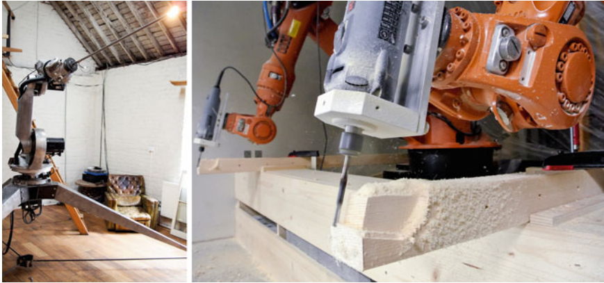
Fig. 1 KUKA KR16 use-cases in the creative industry: Tripod-mounted as part of an art-installation by Conrad Shawcross ( left ), milling wooden elements with an entry-level spindle ( right )
