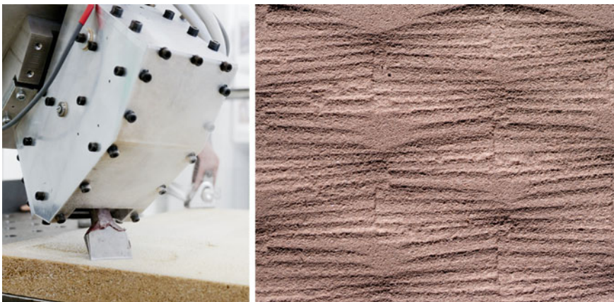
Fig. 3 Dynamic stone surface structuring utilizing the mxAutomation interface to allow dynamic adjustments of angle and force during the structuring process
