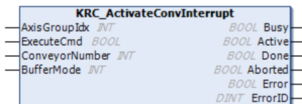
Fig. 6-82: Function block KRC_ActivateConvInterrupt
