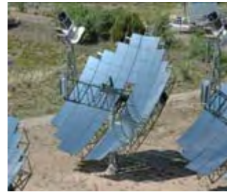
Figure 5.1.3. The Stirling Energy Systems 25-kW dish/Stirling system is undergoing operational testing at Sandia National Laboratories in Albuquerque, NM.
