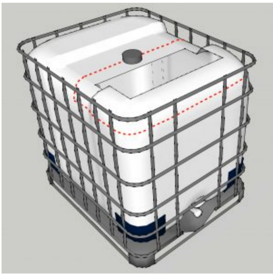
IBC tote or pallet tank showing potential cutaway sections
